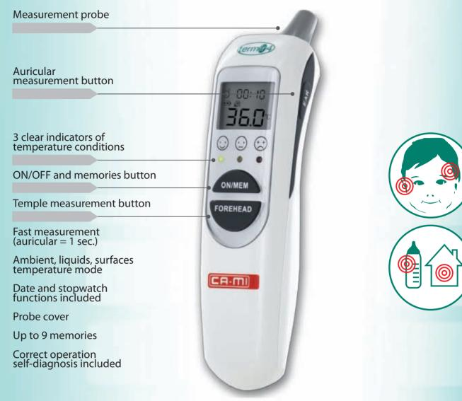
TERMIR-4 is an infrared thermometer with 4 measurement functions: ear, temples, liquids and ambient.
